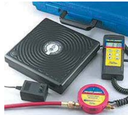
Recharge the system with the exact amount of refrigerant specified on the decal. Recharge either with a recovery unit, an A/C charging station or an electronic weight scale.
