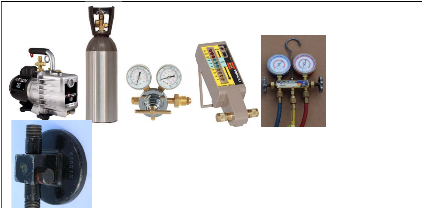
Vacuum pump, nitrogen cylinder, pressure regulator, micron gauge, manifold, dryer made into a bypass
